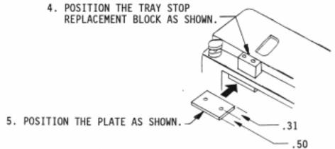
SECURE THE BLOCK TO THE PLATE WITH TWO OF THE SCREWS INCLUDED IN THIS KIT.
